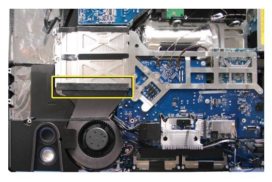
3. Connect the sensor cable and the fan cable to the logic board.
